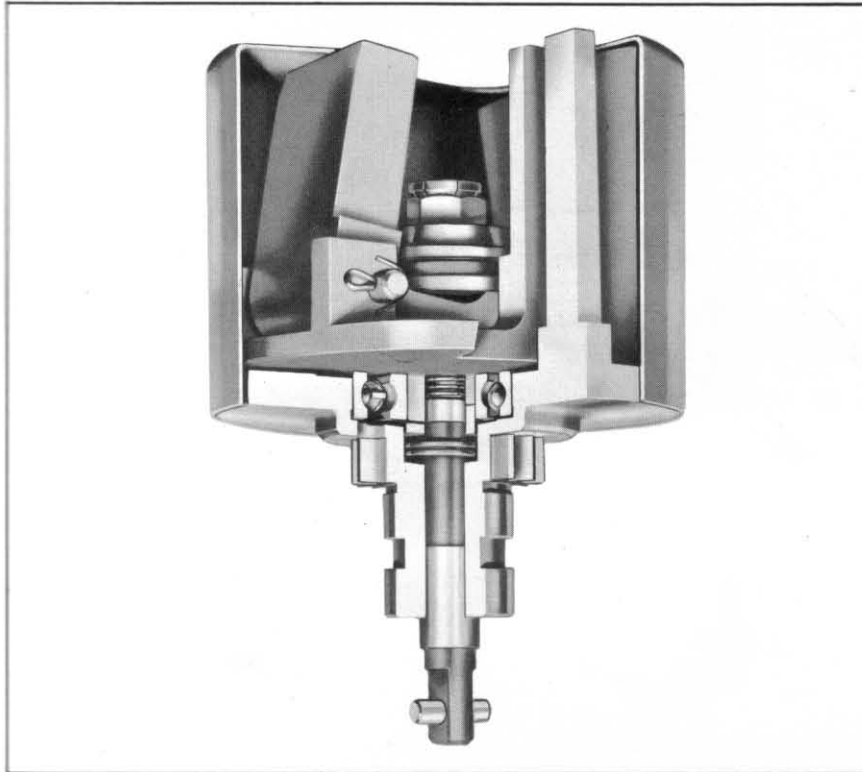
Sectional View of a UG8 Spring Driven Oil Damped Ballhead Assembly
